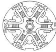
7-way trailer plug car end, rear view
